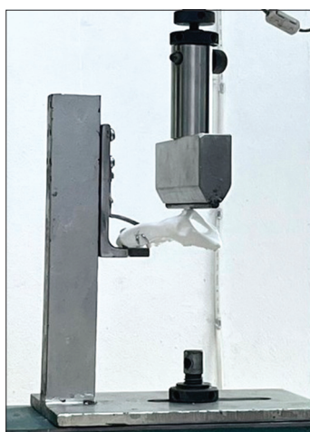
Figure-2: Mechanical loading on the ventral part of a pelvic bone model at the acetabulum level to simulate the physiological loading of the hindlimb in cats.
