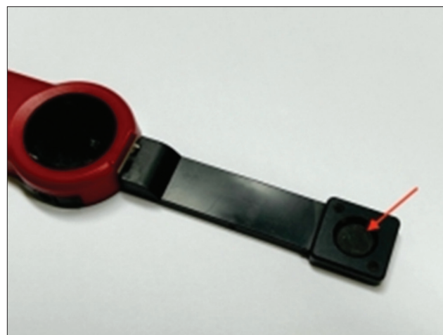
Figure-1: The PM160T wireless thermal power meter is equipped with an ultra-slim sensor that has a diameter of 10 mm (arrow).
