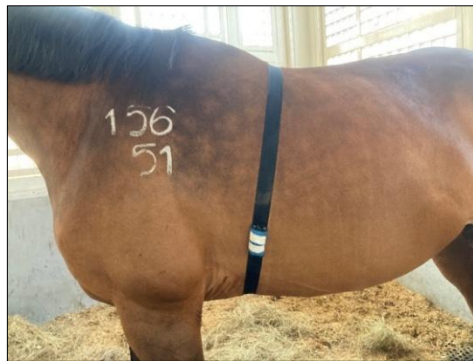
Figure 1: Placement of the heart rate sensor on the horse. The sensor was fastened with a trotter strap behind the withers, with the unit aligned vertically between the shoulder and elbow.
