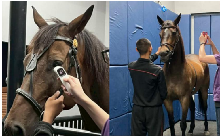
Figure 2: IR positioned to measure temperature at the medial canthus of the eye (left) and TC used to capture thermal images of the horse's head (right). IR = Infrared thermometer. TC = Thermographic camera.
